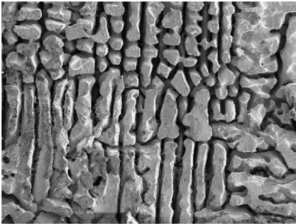
Fig. 14. The corroded Pb–Sb–Cd–(Se)–(Ag) alloy sample.
